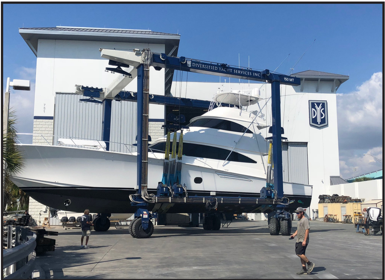
150 M.T. travel lift, paint booth entrance are the grey two-story doors the left.
